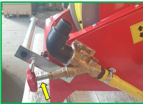
Stopping valve before and during irrigation
